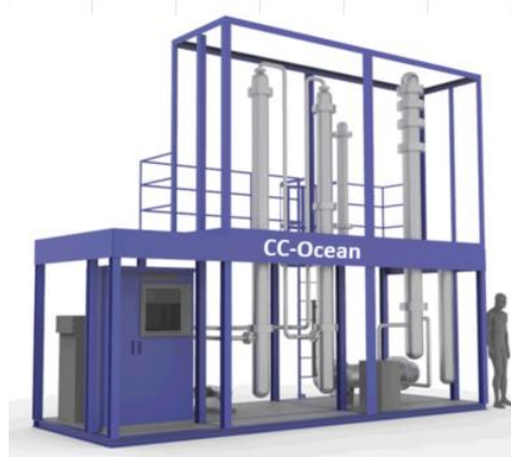
Small-scale CO2 Capture demonstration Plant(image)
